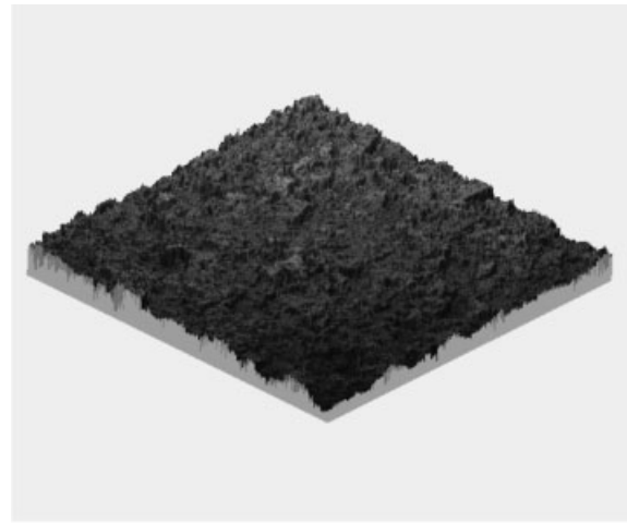
Fig. 7. Eroded surface of the steel X6CrNiTi18-11; parallel projection of the image in Fig. 6
