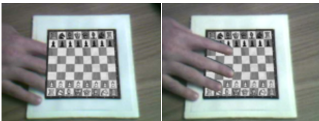
Figure 11 – Visual occlusion correction for the hand using the stencil buffer
