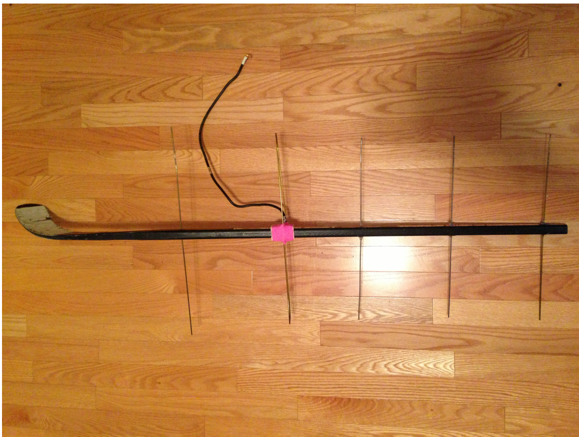
Figure 62: Failed attempt to build an effective Yagi at 315 MHz.
