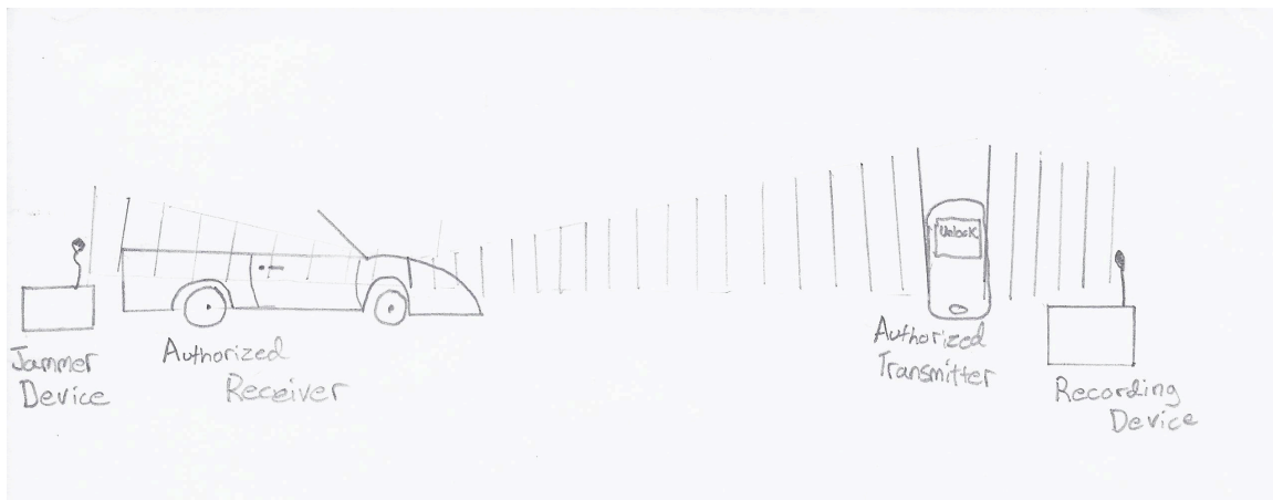
Figure 18: Strategic positioning of the adversary to avoid jamming signal interference.
