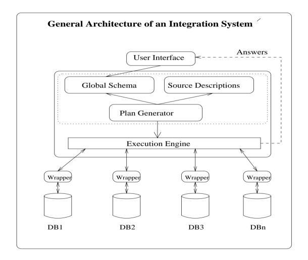
Main components of a mediator-based VDIS
