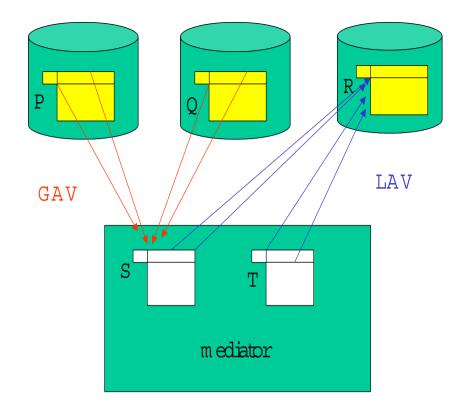
LAV: Mediated schema may contain details than are not in a source
