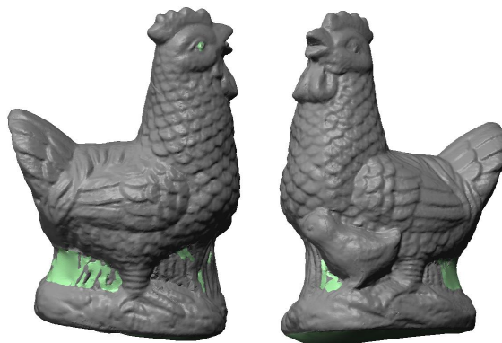
Fig. 13. Holes in chicken scan filled by ReMESH.
