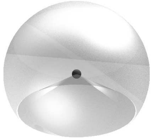
Figure 1: 3D directional antenna of solid angle \Omega = 2\pi(1 - \cos\theta) .
