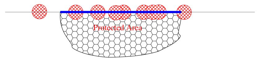
Some sensors move to provide a barrier coverage.
