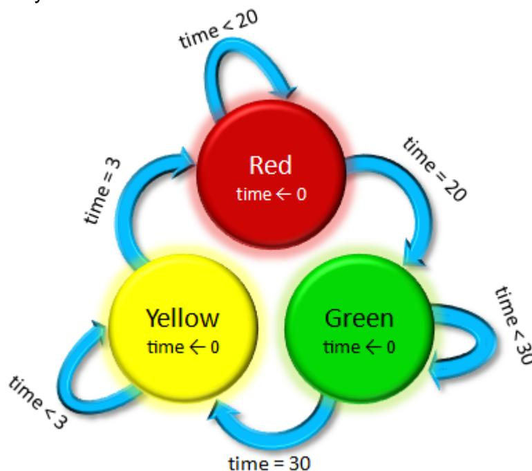
Notice how the state changes from RED to GREEN only when the time has reached 20 seconds. Note as well that inside the state of GREEN, we reset the time counter to 0 so that we can count 30 seconds again in order to decide when to switch to the yellow state.
