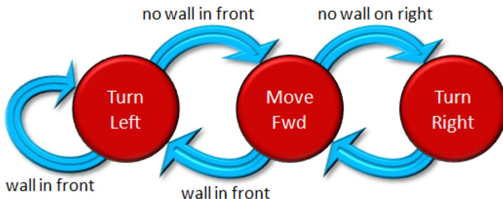
Here is the algorithm, which assumes that each move operation moves the robot one square:
