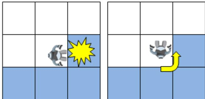
Then the robot should continue moving forwards as it now has its right hand on the wall again. It is possible that while traveling along it may lose contact with the wall →
