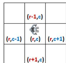
Now, how do we make a turn? Turning does not change the location of the robot, it just changes the direction. Let's assume that each turn makes a 90 degree change in direction (e.g., from EAST to NORTH or from EAST to SOUTH, but never from EAST to WEST).
