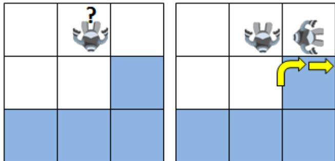
In this case, notice that the robot needs to regain contact again with the wall on its right. First, it must turn right. However, the wall will still not be on the right of the robot after turning. Therefore it also needs to move forward.
