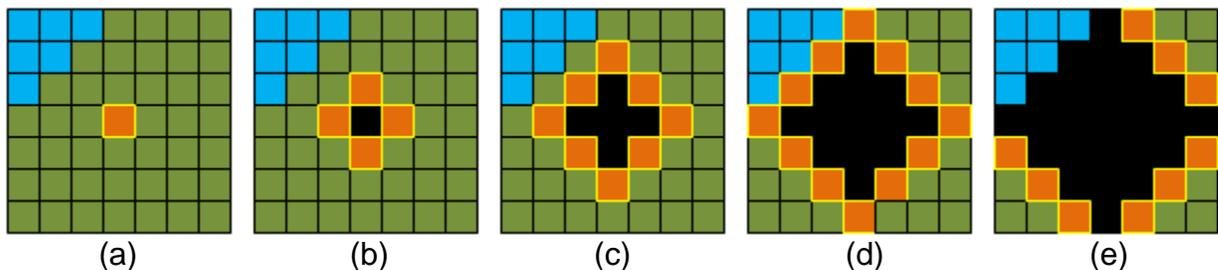
Notice that as the fire spreads ... there is a "wall" of fire that expands outwards, while the interior burned portions remain black. Intuition again tells us that we only need to consider this "wall" (also known as the **active border**) of the fire in order to determine the spread-pattern of the fire. That is, each orange pixel is itself a kind of *miniature fire* that needs to be spread outwards.
