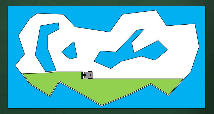
One approach is to simply travel in some fixed direction (e.g., North) until an obstacle is encountered, then turn around...cover in strips:
