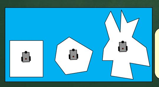
With limited direction capabilities, robot would have to rotate to view entire environment
