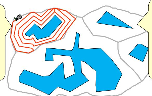
This technique is best for robots that have dead-reckoning errors. By maintaining fixed distance from obstacle, robot can readjust its measurements and re-confirm its position.
