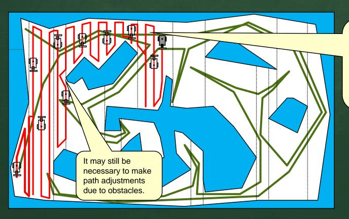
Usually, vertical motions up and down separated by a robot width. Such motions are joined by travel along the obstacle boundary.
