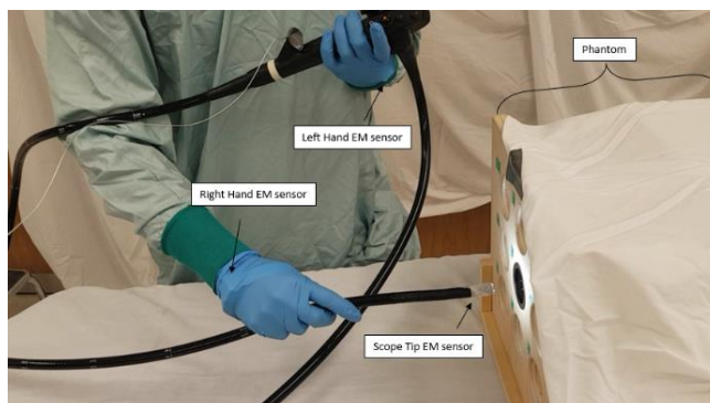
Figure 2. Experimental setup; shows three sensors, a covered phantom, and a participant
