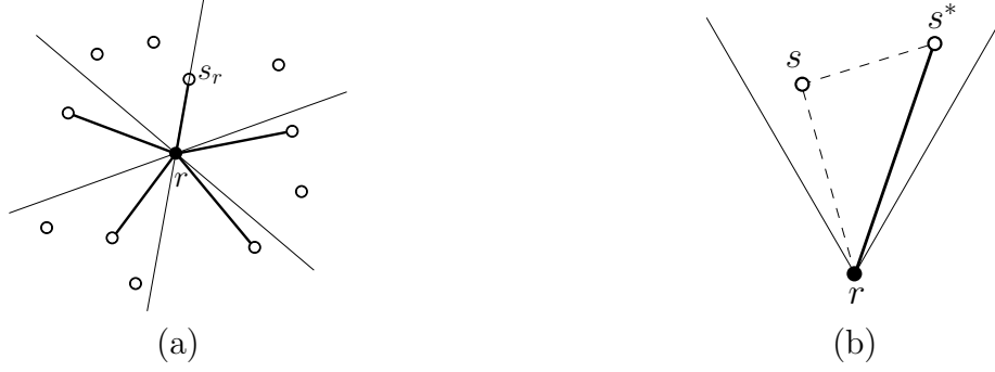
Figure 3: (a) s_r is the nearest neighbor of r which is shared between two cones; bold edges are added to G' . (b) The edge (r, s^*) \in T_{opt} is replaced by two edges (r, s) and (s, s^*) .
