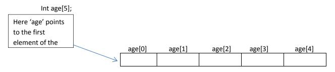
In C, name of the array always points to the first element of an array. Here, address of first element of an array is &age[0]. Also, age represents the address of the pointer where it is pointing. Hence, &age[0] is equivalent to age. Note, value inside the address &age[0] and address age are equal. Value in address &age[0] is age[0] and value in address age is \*age. Hence, age[0] is equivalent to \*age.
