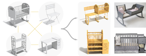
Fig. 1: Starting from a heterogeneous collection of four objects (left) as initial population, our functionality-aware evolution tool can generate a variety of plausible hybrid shapes. Two of them (middle) exhibit strong functional similarity to exiting professional designs (right).
