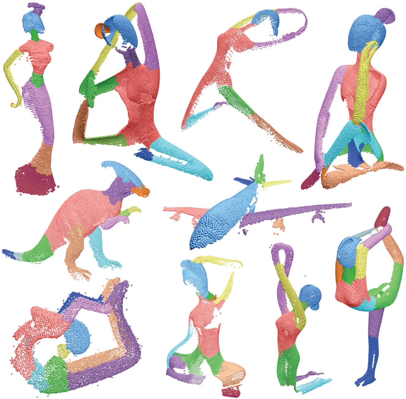
Fig. 5: Segmentations obtained with our non-parametric algorithm on a collection of point clouds acquired with a range scanner.
