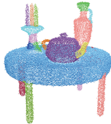
Fig. 10: A point cloud corresponding to an indoor scene with multiple objects, segmented with our method.
