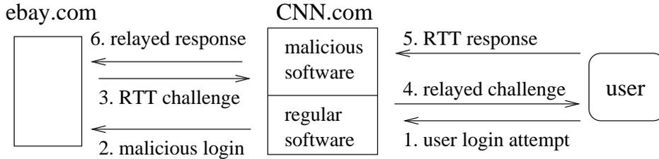
Fig. 4. ATT Relay Attack
