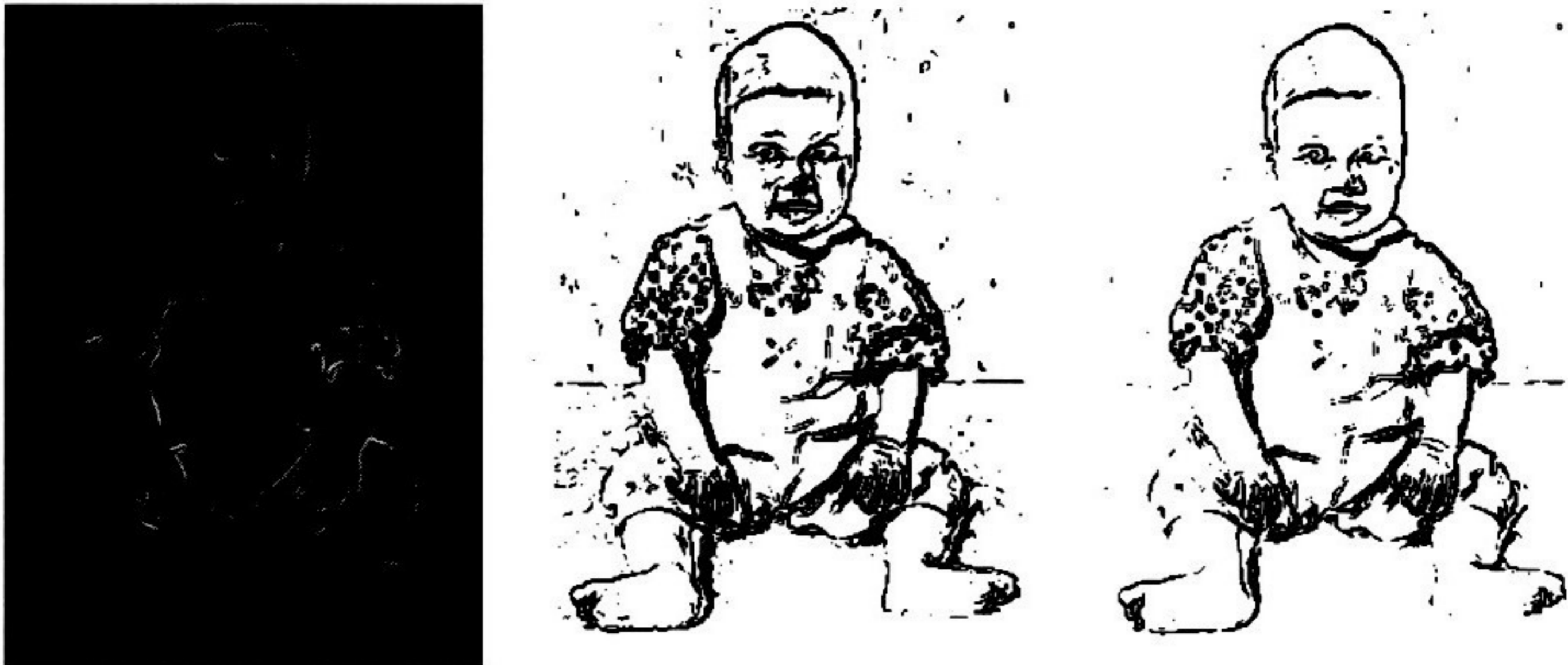
Figure 4.7 Left: output of Sobel edge enhancer run on Figure 4.1. Middle: edges detected by thresholding the enhanced image at 35. Right: same, thresholding at 50. Notice that some contours are thicker than one pixel (compare with Figure 4.5).
