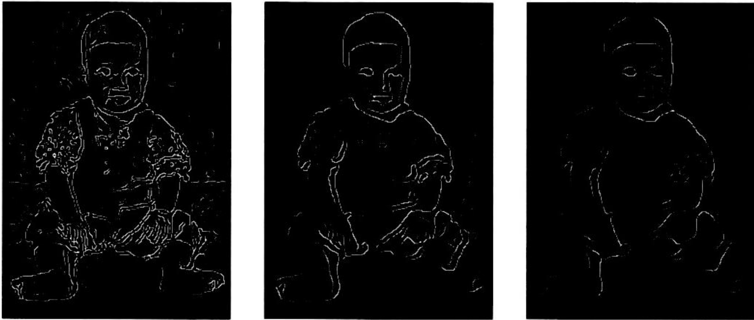
Figure 4.5 Strength images output by CANNY_ENHANCER run on Figure 4.1, after nonmaximum suppression, showing the effect of varying the filter's size, that is, the standard deviation, \sigma_f , of the Gaussian. Left to right: \sigma_f = 1, 2, 3 pixel.
