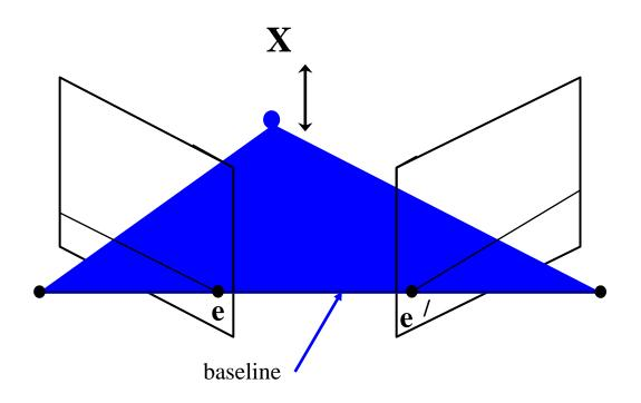
As the position of the 3D point  $\mathbf{X}$  varies, the epipolar planes "rotate" about the baseline. This family of planes is known as an epipolar pencil. All epipolar lines intersect at the epipole.
