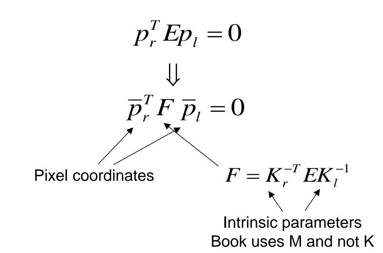
Mapping between points and epipolar lines in the pixel coordinate systems
