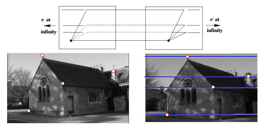
Epipolar geometry depends only on the relative pose (position and orientation) and internal parameters of the two cameras, i.e. the position of the camera centres and image planes. It does not depend on the scene structure (3D points external to the camera).
