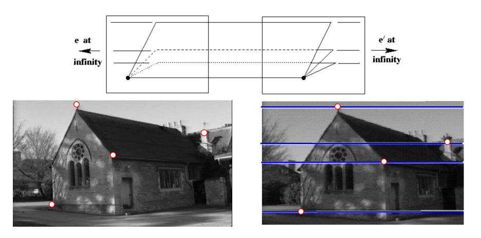
Epipolar geometry depends only on the relative pose (position and orientation) and internal parameters of the two cameras, i.e. the position of the camera centres and image planes. It does not depend on the scene structure (3D points external to the camera).
