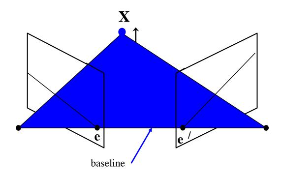
As the position of the 3D point X varies, the epipolar planes "rotate" about the baseline. This family of planes is known as an epipolar pencil. All epipolar lines intersect at the epipole.
