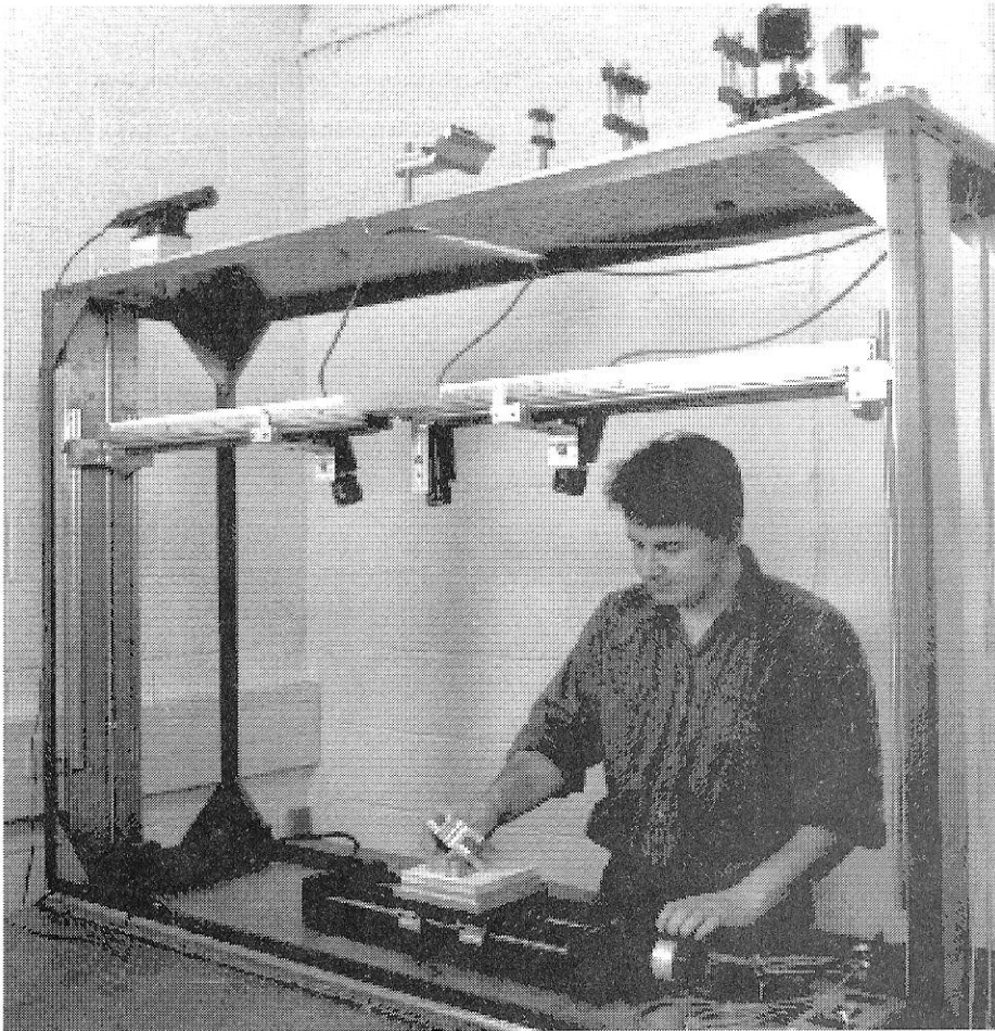
Figure 2.16 A real 3-D triangulation system, developed at Heriot-Watt University by A. M. Wallace and coworkers. Notice the laser source (top left), which generates a laser beam; the optical components forming the plane of laser light (top middle and left); the cameras; and the motorized platform (bottom middle) supporting the object and sweeping it through the stationary plane of light.
