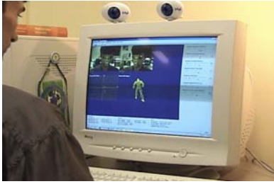
Figure 1: Stereo tracking with two web-cameras. The key issue is finding the relationship between the cameras.
