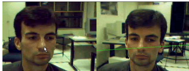
Figure 3: Learning the features using the epipolar constraints. The nose feature must lie on the epipolar line.
