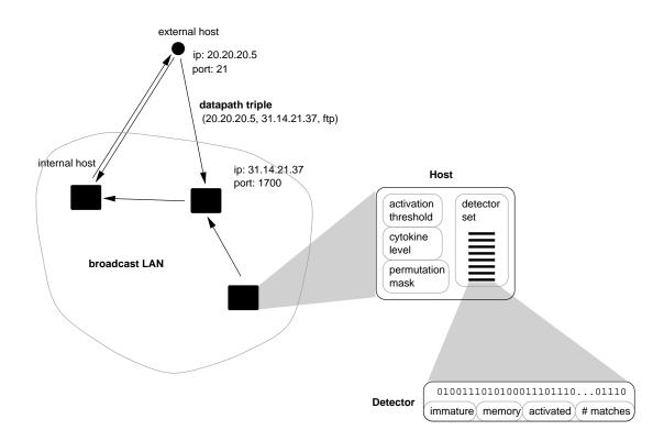
Figure 1: The Architecture of the AIS.
