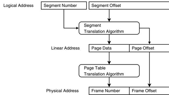
Figure 6. Translation from virtual to physical addresses on the x86
