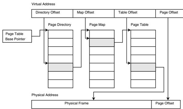
**Figure 3. Translation of a Virtual to Physical Address through Page Tables**
