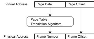
**Figure 2. Translation of a Virtual Address into a Physical Address**
