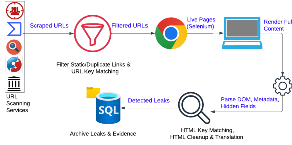
Figure 1: Leak Detection Workflow Overview
