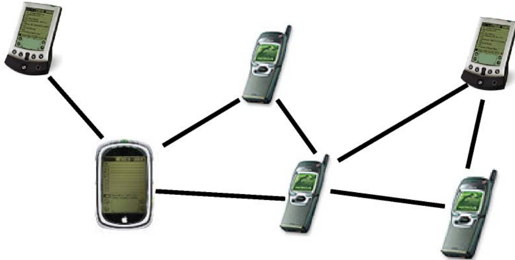
Figure 20: Self-organized ad hoc wireless network
