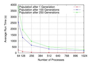
Figure 5: Runtime results for InSiPS worker process benchmarking test on the Scinet BGQ cluster.
