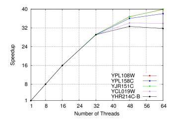
Figure 4: Speedup results for InSiPS threads/worker benchmarking tests on the Scinet BGQ cluster.
