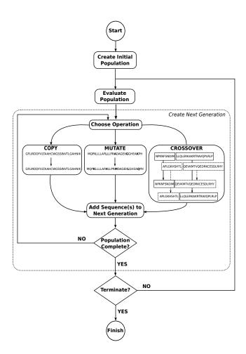
Figure 1: Graphical overview of the core InSiPS genetic algorithm.
