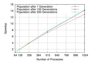
Figure 6: Speedup results for InSiPS worker process benchmarking test on the Scinet BGQ cluster. 64 nodes was the minimum job size and is thus used as a baseline. A speed-up of 16x using 1024 nodes would represent linear speed-up in this scenario.
