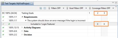
8. In the *Test Targets* view, click on the column number 1 (i.e. the first test case). The test will be selected and shown as message sequence diagram. The model browser will show how the test is exercising the model.
