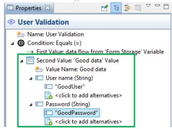
When generating tests, Creator will gather all data stored in the variable and compare it against the values that are added into the *Second Value* (*Good data*) item. If the data from the variable equals/matches *Good data*, Creator will create a test covering the "yes" branch. In other cases Creator will create a test case covering the "no" branch.
