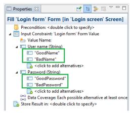
Note: A user has also option to specify data coverage conditions. This option occurs only when value lists or alternate input values are specified. The options of the data coverage are shown below.
