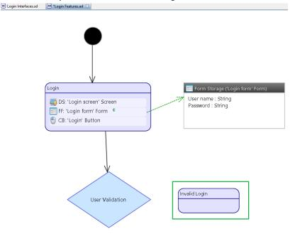
4. Add a *Control Flow* form *User Validation* decision diamond to *Invalid Login* activity. Once the *Control Flow* from a Decision is drawn, user needs to choose which path will be associated with the *Control Flow*. Choose *Create False Control Flow* (N).
