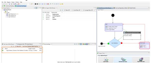
As it can be observed on the right side of the picture above, the *Model Browser* shows that the no branch of the *User Validation* decision diamond has not been covered, hence the path along with the *Invalid Login* activity has being marked in red. This usually means that either there is something wrong with the model or that Conformiq Creator needs higher lookahead depth. For more information on lookahead depth, please refer to the Conformiq Creator user manual.
