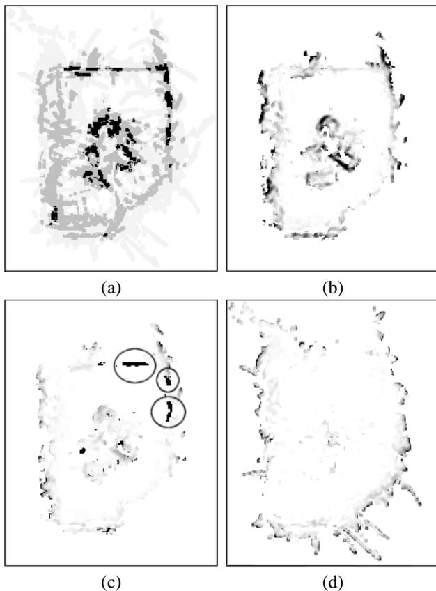
Figure 9. (a) Grid cell weight classification, (b) Combined data with single sensor readings removed, (c) Vision data combined with Sonar/IR data showing where gaps were filled in, (d) Noise that was eliminated from the vision data.
