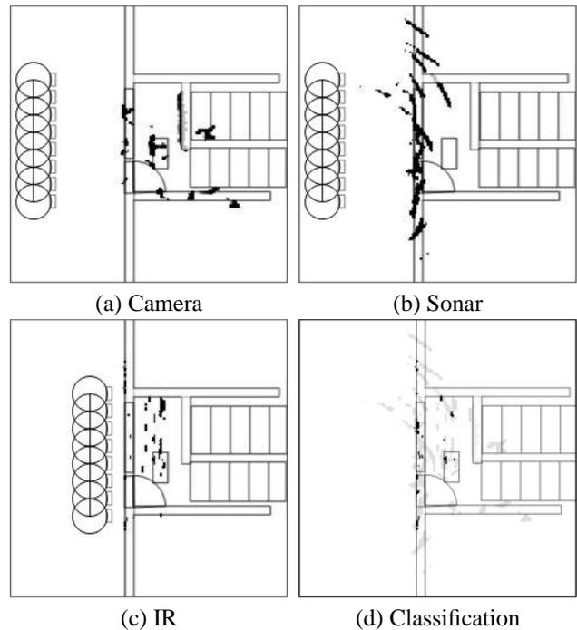
Figure 6. Range data from the window/stairwell test.
