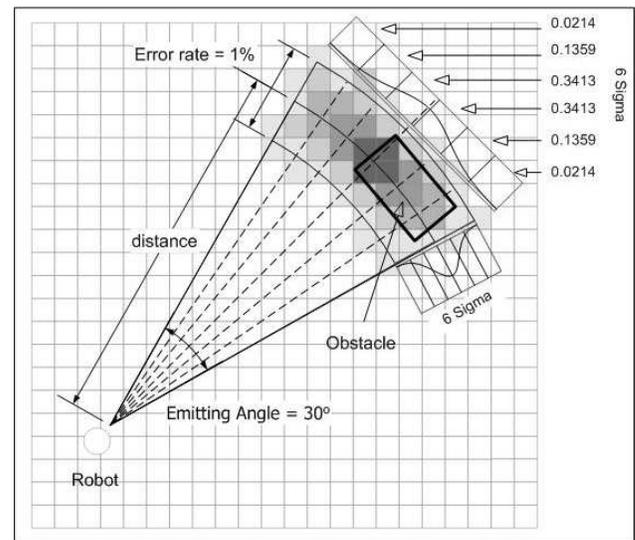
Figure 3. Diagram showing the occupancy grid cells that need to be updated during a single sonar reading.
