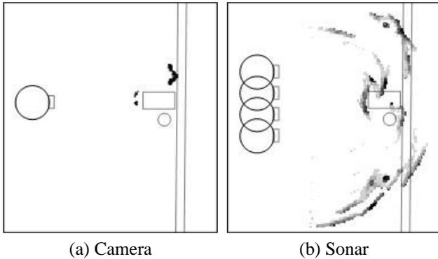
Figure 7. Range data from the low lighting test.
