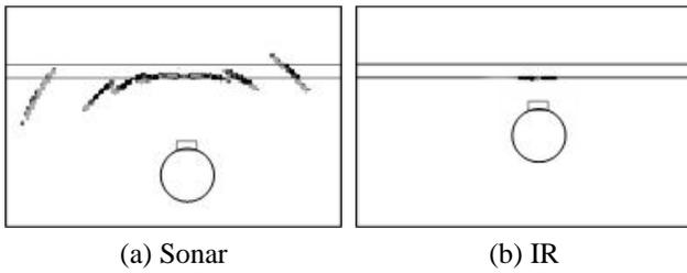
Figure 4. Range data from the blank wall test.
