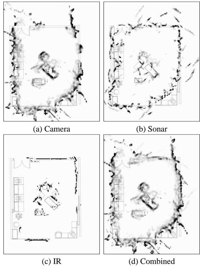
Figure 8. Range data from the full lab test.
