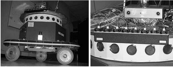
Figure 1. The robot used for testing and a closeup view showing the BumbleBee stereo camera, infrared proximity sensors and sonar ring.
