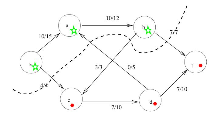
Capacity of Cut= 4 + 3 + 7 = 14Net flow across the cut= 4 + 3 + 7 - 0 = 14
