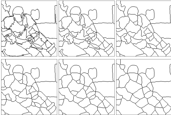
Figure 4: The original image, then openings with erosion masks of radius 4, 6, 8, 10, 12.
