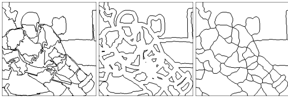
Figure 1: Region smoothing. Original region boundaries, left; the eroded region boundaries, middle; and the completely opened regions, right.
