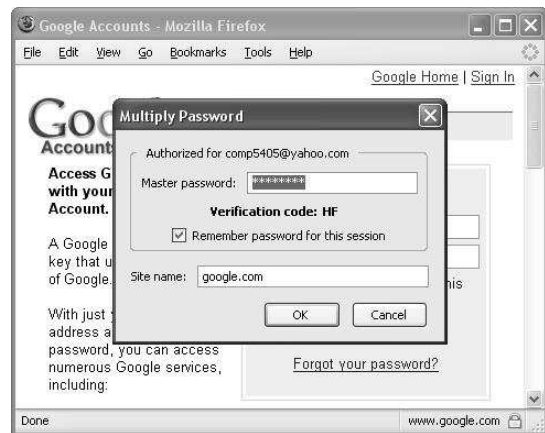
Figure 2: The dialog box for P-Multiplier is activated by double-clicking on the password field
