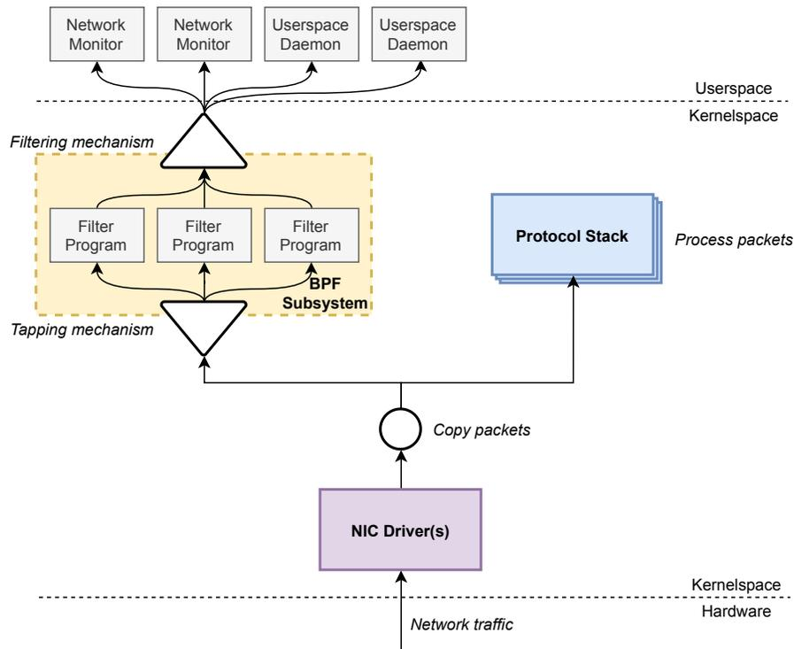
**Figure 2.7:** The classic BPF architecture. A tap intercepts and copies packets as they arrive from the NIC driver before they are forwarded to the operating system’s protocol stack. The tap then passes packets through a filtering mechanism which selectively delivers them to various consuming userspace applications. This figure was adapted from McCanne and Jacobson [98].
