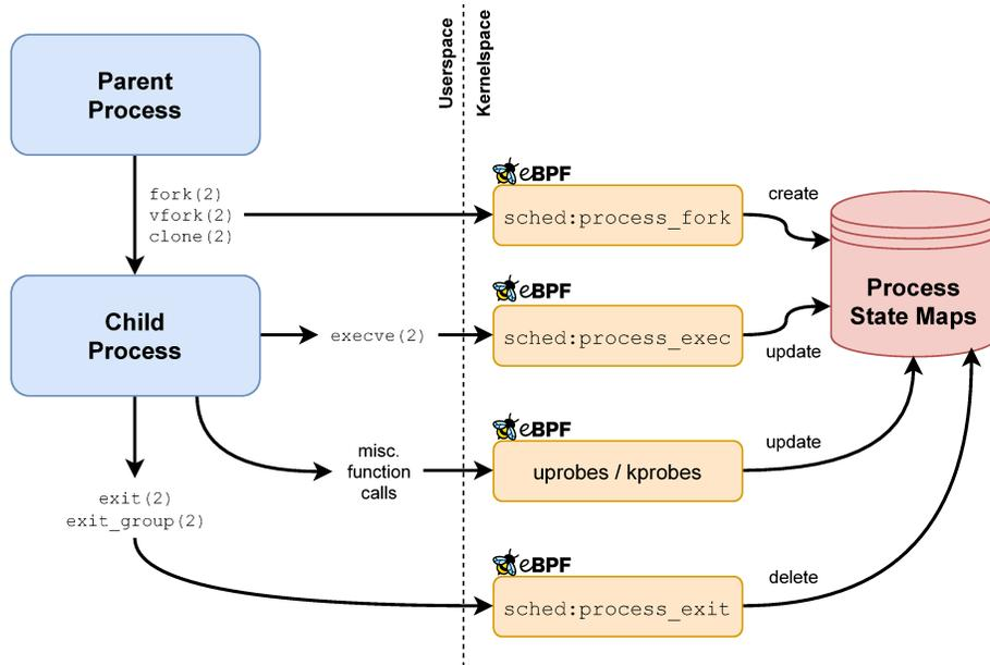
**Figure 4.2:** The various mechanisms that BPFBOX uses to manage process state. Probes marked `sched:*` are tracepoints instrumenting scheduler events in the kernel. Uprobes and kprobes instrument userspace and kernelspace function calls respectively.
