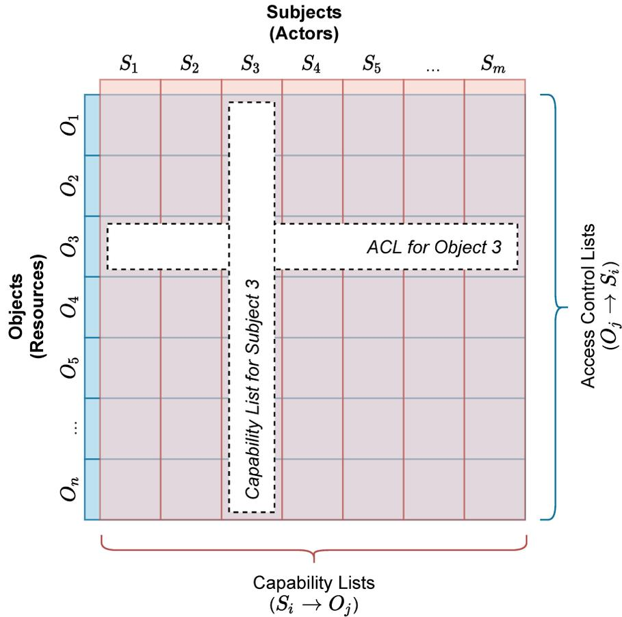
**Figure 2.3:** The access matrix and the relationship between ACLs and capability lists [2, 75, 107]. ACLs define the set of subjects that have specific access rights on a particular object. Capability lists conversely define the access rights that a specific subject has on a set of objects. Note that an ACL may be derived by taking the set of all capability lists and vice versa. Taken together, these form the access matrix.
