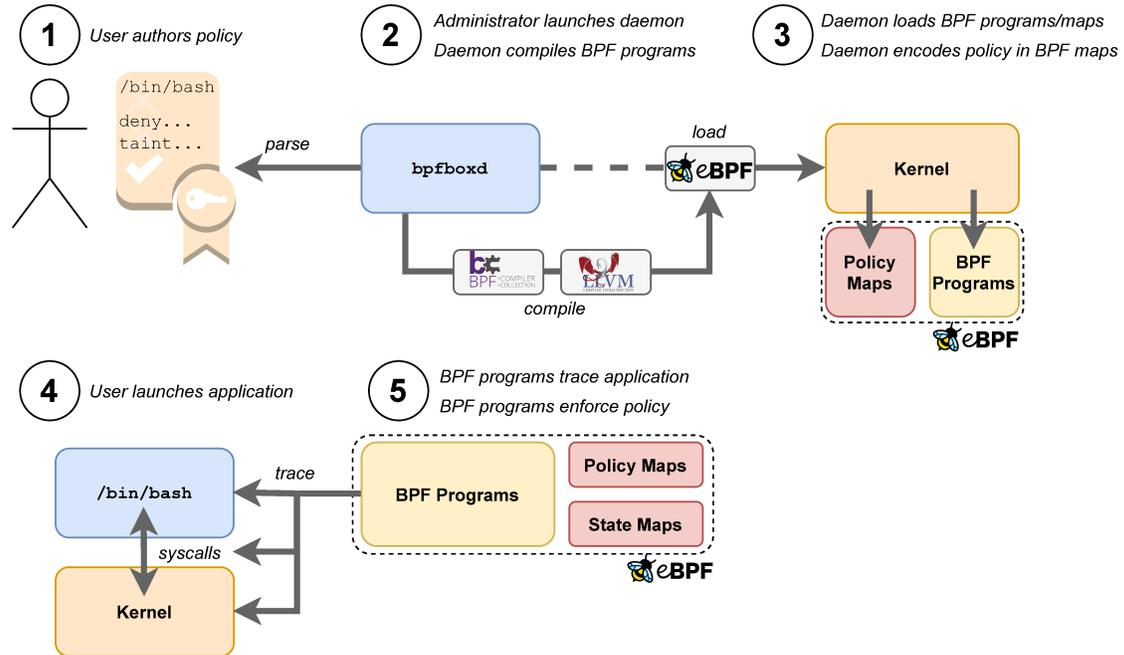
**Figure 4.1:** A high-level overview of how BPFBOX confines applications. Users write policy files which the daemon encodes into eBPF maps. Using the `bcc` toolchain for Python, the daemon compiles and loads its eBPF programs and maps into the kernel. At runtime, BPFBOX’s BPF programs trace the application and enforce security policy by querying the state stored in its maps.
