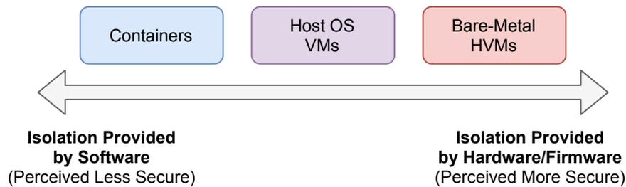
**Figure 3.1:** Comparing the isolation and perceived security of containers and VMs. A boundary defined in hardware is often considered more rigid, whereas a software defined boundary is generally considered more malleable, and thus weaker. However, this need not be the case. A goal of this thesis is to improve the security of containers by hardening the boundary between the container and the host operating system.
