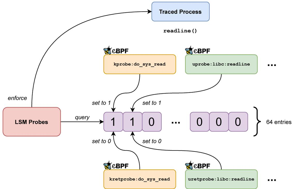
**Figure 4.3:** How BPFBOX uses kprobes and uprobes to track function calls. If a policy identifies that a rule should apply within the context of a certain function call, BPFBOX instruments a probe on function entry and return. These probes flip the corresponding bit in the process’ state vector, indicating to policy enforcement probes whether or not the process is in the middle of making the function call.
