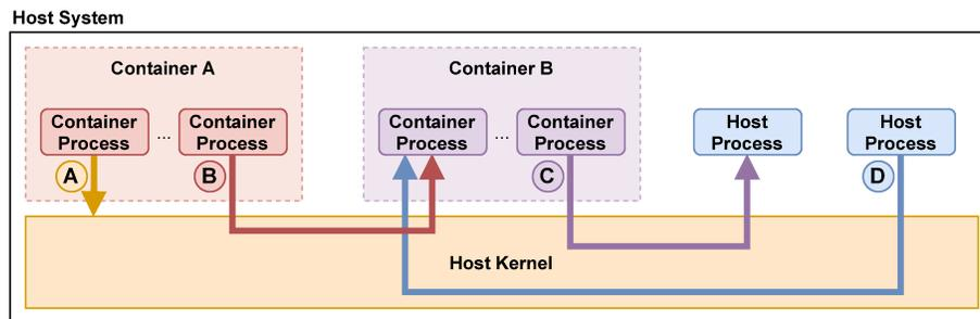
**Figure 2.6:** A sample threat model for container security. (A) A container process attacks the host kernel directly. (B) A container process attacks another container process, passing through the host kernel’s reference monitor. (C) A container process attacks a (privileged) host process, passing through the host kernel’s reference monitor. (D) A host process attacks a container, passing through the host kernel’s reference monitor.
