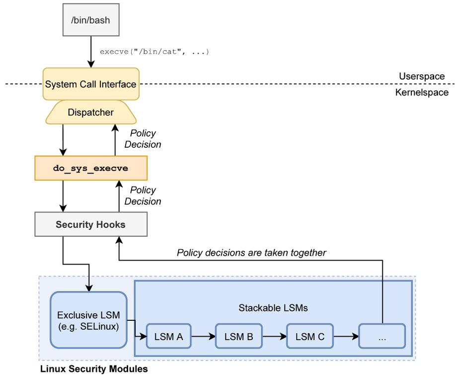
**Figure 2.4:** The LSM architecture. A single *exclusive* LSM may be loaded at a time, and complemented by zero or more *stackable* LSMs. When userspace requests a privileged operation (e.g. through a system call), this operation causes one or more security hooks to be invoked. These hooks in turn call into the respective hook implementations provided by each loaded LSM. Each hook returns a policy decision, and these decisions are then taken together to arrive at a final decision.
