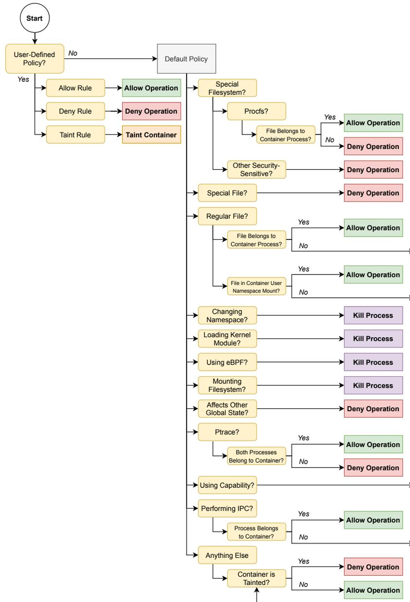
**Figure 5.2:** The policy enforcement strategy under BPFCONTAIN, expressed as a flowchart. Using container semantics, BPFCONTAIN achieves rich policy defaults, denying access to global resources and operations which can affect global system state while preserving intra-container access. This greatly simplifies the resulting confinement policy and enables the user to focus on specific exceptions to default protection.
