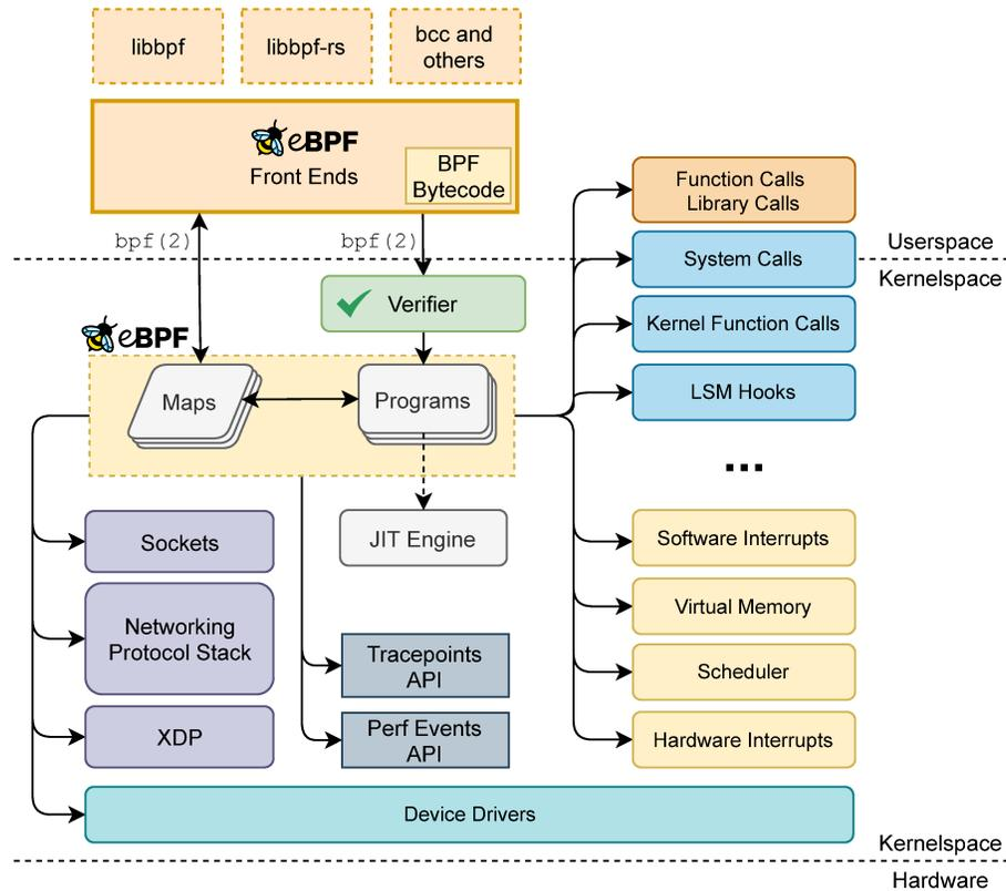
**Figure 2.8:** The extended BPF architecture. Unlike classic BPF, eBPF programs are JIT (Just-In-Time) compiled to the native instruction set, share data using specialized map data structures, and can be attached to many different kinds of system events. Programs can share data with each other and with the controlling userspace process using specialized map data structures. All eBPF bytecode goes through a verification step before it can be loaded into the kernel.
